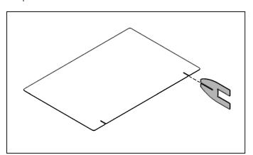
**STEP 3:** Slide Cubicle Wall Adapter into slot on Main Panel. Take remaining Adapter and slide into slot on other side of Panel.
