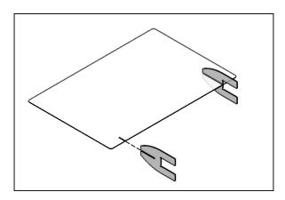
step 4: With one person holding each end of your assembled Wall Extender and supporting the Adapters underneath, stand unit upright and guide down over top of cubicle walls.
