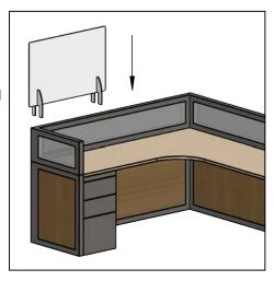
NOTE: For installing units with 3 Adapters, install your Cubicle Wall Extender with two adapters as noted in STEPS 2-4, then angle one side of your installed unit up slightly and slide in the third Adapter to lock into middle position slot.
