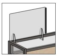
**STEP 6:** Guide your additional Cubicle Wall Extender down over cubicle wall and then align with open end of Flexible Connector. Connect units together by inserting edge of Panel into Connector.
